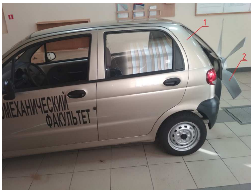
Figure 5. The vehicle equipped with an air propeller: 1– vehicle; 2 - air propeller.
