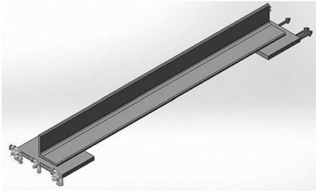
Fig. 3. Scheme of fastening and loading joints of an angle bar with a gusset.
