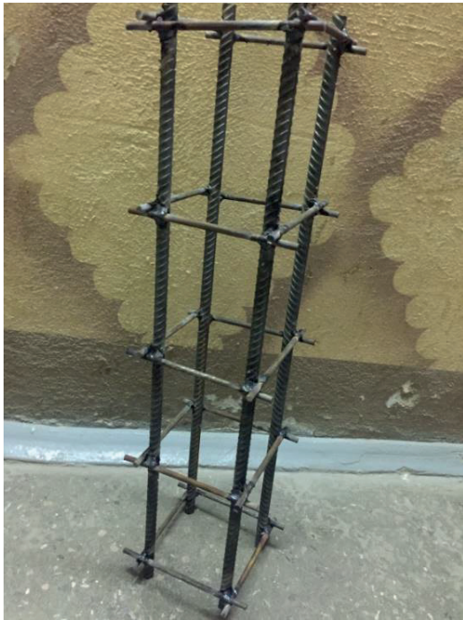
Figure 1. Spatial reinforcement cage for manufacture of specimens
