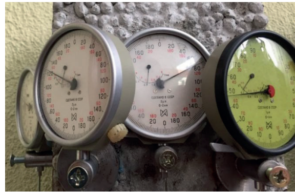
Figure 4. Dial-type indicators installed into steel adapter points to record shrinkage strain of expanded clay concrete and stain of longitudinal reinforcement
