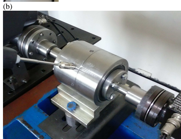
Fig. 4. Speed reducer casing temperature measurement: (a) a pyrometer with contact probe (Testo 830-T2 model); (b) measurement of the speed reducer casing temperature on the test bench
