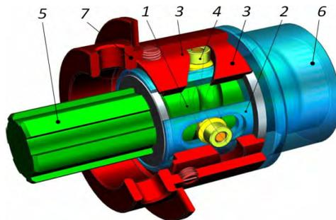
The inner and outer cams and the cage form a three-link mechanism with the kinematics which is similar to the kinematics of a planetary gear. One link is a driving one, the second link is a driven one, and the third link is a fixed one during reducer (multiplier)
