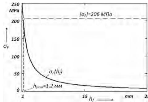
The maximum flexural stress occurs at the top of the lobe, which may cause its breakage. At the same time, the height of the lobe section  $h_{f\min}$ , where the calculated stress exceeds the allowable ones is negligible (Figure 4). This section can be cut off during manufacture. The height of the cut-off section is calculated by the formula:
