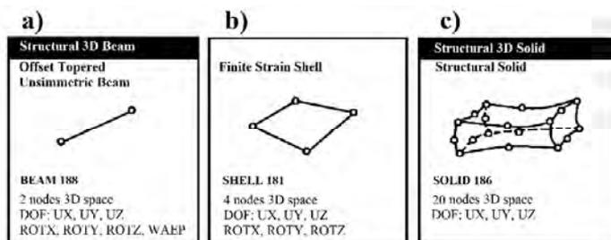
Figure 1. The finite elements used in the study.
